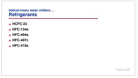
Manufacturers are continuously improving their designs of helical-rotary water chillers. New chillers need to be designed around the characteristics of the refrigerant. Today there are 5 strong candidates for use with positive-displacement, helical-rotary chillers. They are HCFC-22, HFC-134a, HFC-404a, HFC-407c and HFC-410a.
